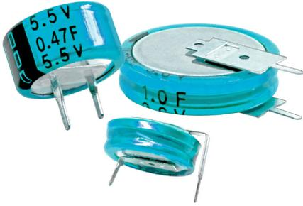
Type EDC electric double layer supercapacitors offer high capacitance values in a thru hole stacked coin type package. Primarily designed for integrated circuit voltage backup, the capacitors can also be used to deliver the initial power from batteries.
