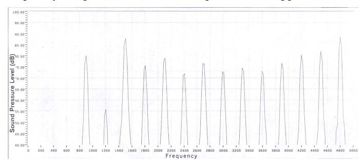
As shown above, the fundamental frequency is below 1 kHz, and there are more than 4 harmonic peaks between 1 and 4 kHz. All harmonic peaks are within  $\pm$  15 dB of the fundamental frequency.
