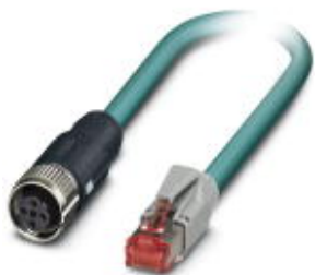
Network cable, Ethernet CAT5 (100 Mbps), 4-position, PUR, water blue RAL 5021, shielded, Plug straight RJ45 / IP20, on Socket straight M12 SPEEDCON / IP67, coding: D, cable length: 1 m
