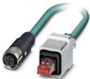
Network cable, Ethernet CAT5 (100 Mbps), 4-position, PUR, water blue RAL 5021, shielded, Plug straight RJ45 Push Pull / IP67, on Socket straight M12 SPEEDCON / IP67, coding: D, cable length: 2 m
