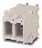
Contact insert, Contact insert, housing material: PA 6.6, number of positions: 2, nom. voltage: 400, rated current: 20 A, Type of contact: Pin. Connectors may only be connected/disconnected when under no load.
