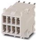
Contact insert, Contact insert, housing material: PA 6.6, number of positions: 8, nom. voltage: 160, rated current: 10 A, Type of contact: Pin. Connectors may only be connected/disconnected when under no load.
