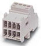
Contact insert, Contact insert, housing material: PA 6.6, number of positions: 8, nom. voltage: 160, rated current: 10 A, Connection method: Screw connection, Type of contact: Pin. Connectors may only be connected/disconnected when under no load.
