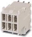
Contact insert, Contact insert, housing material: PA 6.6, number of positions: 6, nom. voltage: 250, rated current: 10 A, Type of contact: Pin. Connectors may only be connected/disconnected when under no load.
