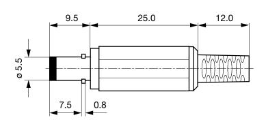
Cable diameter max. 4.0 mm
