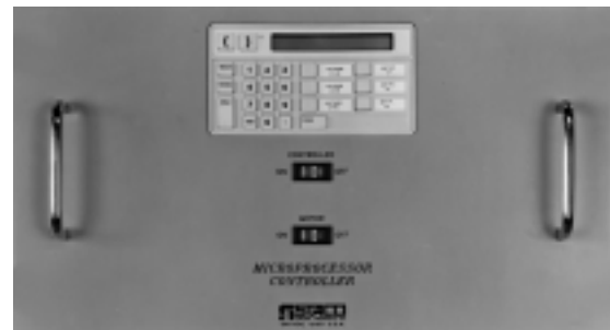
Figure 5. MP Control Panel
